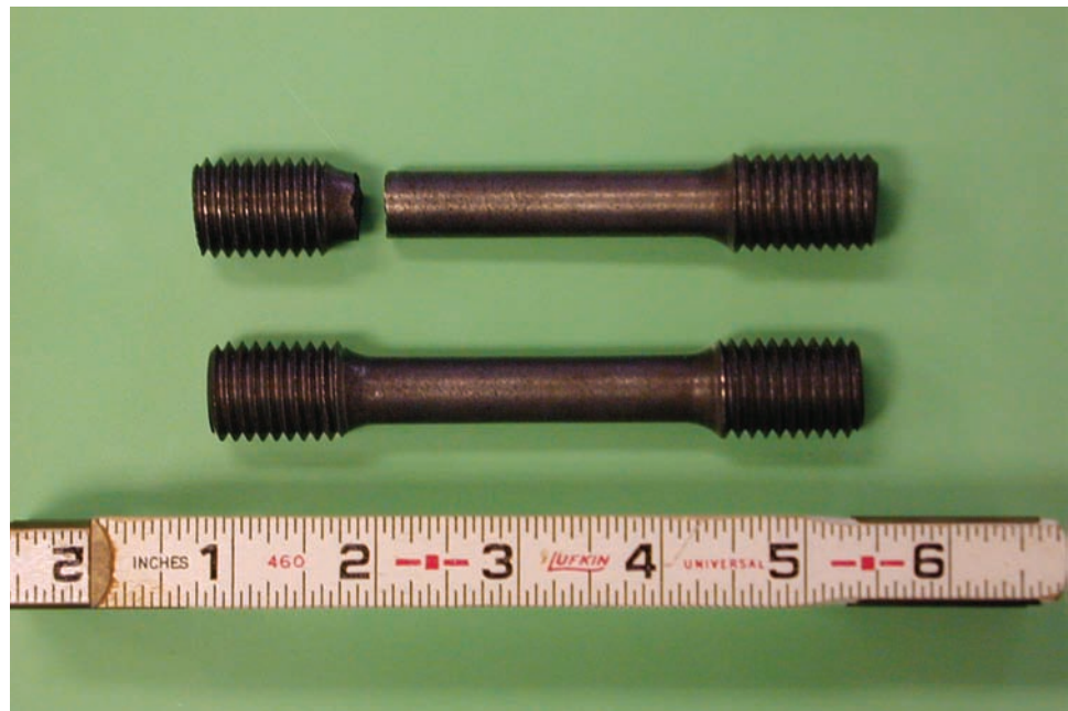
Figure 8.1.9 Brittle Fracture of Cast Iron Specimen
